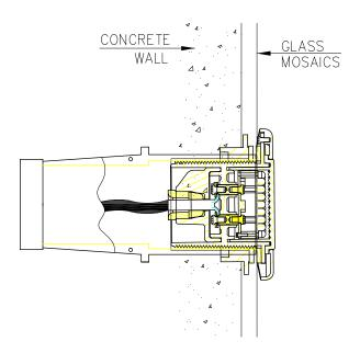
Prior to concreting, place a ¾" threaded female adaptor 500-700mm below water surface level, making sure the face of the adaptor is fixed flush against the future finished wall level of your pool interior. This socket will be used for fixing the underwater gland (provided) for a watertight installation.
