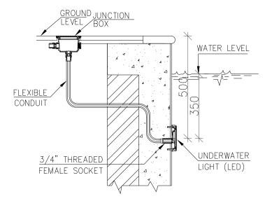
Prior to concreting, place a 3/4" threaded female adaptor 500-700mm below water surface level, making sure the face of the adaptor is fixed flush against the future finished wall level of your pool interior. This socket will be used for fixing the underwater gland (provided) for a watertight installation.
